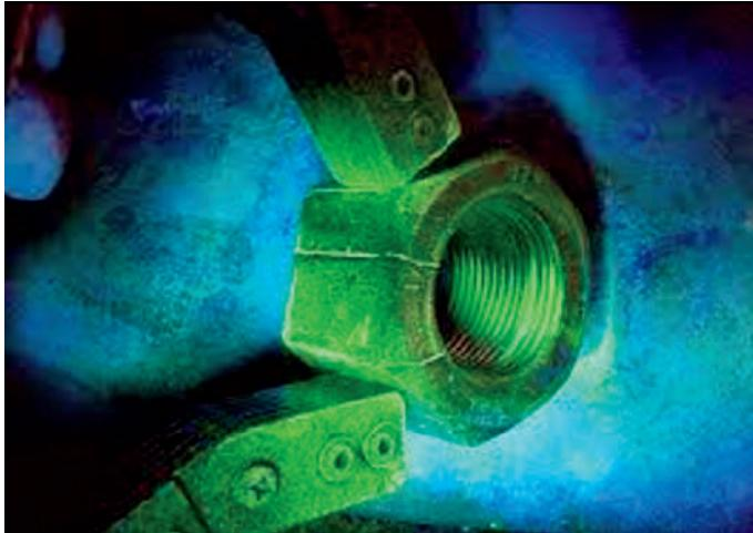
Magnetic particle testing (MT) is a nondestructive testing (NDT) method for detecting surface and shallow subsurface discontinuities in ferromagnetic materials such as iron, nickel, cobalt, and some of their alloys.
