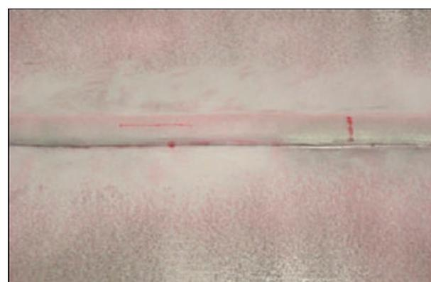
PT is intended to detect surface breaking flaws such as cracks, laps and porosity.
